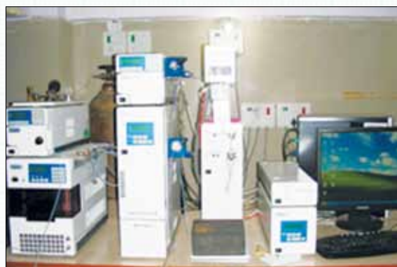
Supercritical Fluid Extraction
