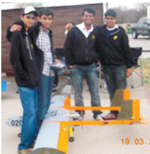
Twin Boom Pusher configuration aircraft design. Much appreciated by judges at the SAE event.
