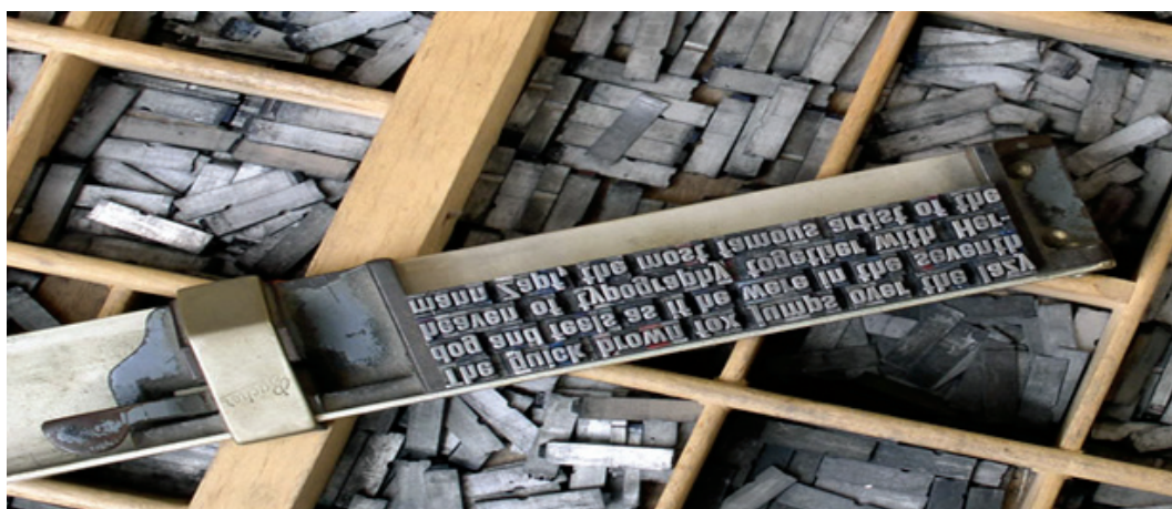
Movable Type and a Plate of Assembled Characters
