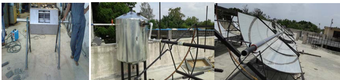
Fabricated Mobile Blancher unit for Turmeric processing and Steam Water Separator with Insulation Cover and CPC Panels
