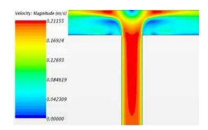
**Figure 1:** Tee junction dividing flow simulation
