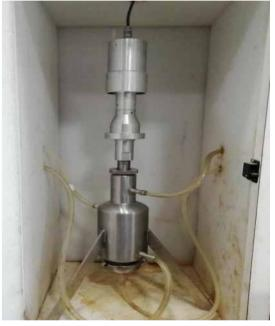
**Ultrasonic Continuous flow cell**
