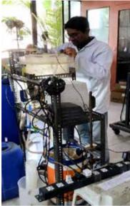
Pulsed Disk and Doughnut Extraction Column Setup
