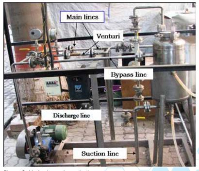
Figure 2: Hydrodynamic cavitation setup
