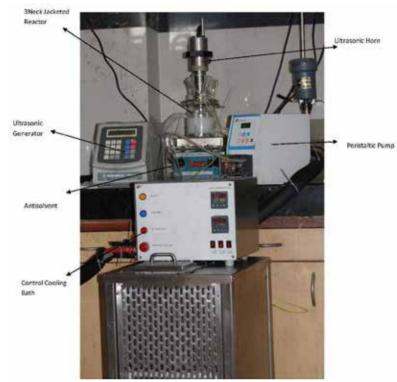
Figure 1: Anti solvent crystallization setup
