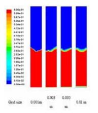
**Figure 3:** Contours of volume fraction of solids in Fluidized Bed
