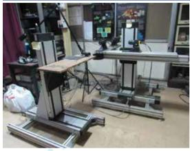
Farticle Image Velocimetry Setup
