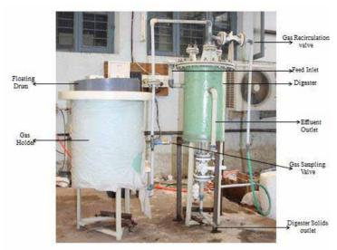
Figure 3: Biogas generation from food waste
