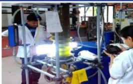
Pulsed Disk and Doughnut Extraction Column Setup
