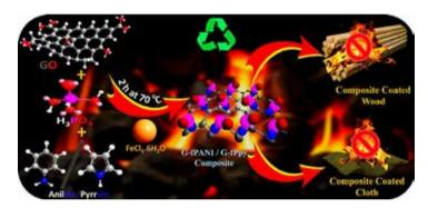
**Scheme 1:** Synthesis of Polymer-Functionalized Graphene Composite Flame Retardant (G-fPANI and G-fPPy)
