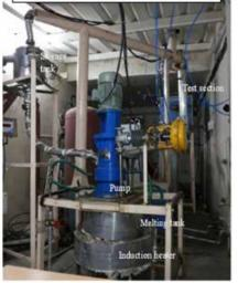
Molten Salt Heat Transfer Loop
