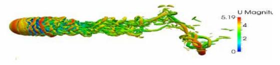
Figure: Velocity iso-contours for flow past a sphere obtained from fully resolved DNS implemented on a hexahedral mesh configuration of 128 Million cells, using a second order accurate central differencing scheme.
