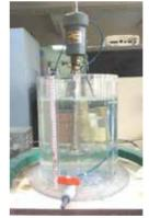
Fig 1. Experimental setup of the stirred tank Fig reactor (6-blade Rushton turbine) plo
