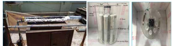
Figure 1: Thermal diode receiver experimentation under the sun.
