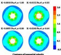
Fig 2. Contours plots of the tangential velocity plotted on the XZ plane (6-blade Rushton turbine)
