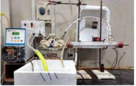
*Fig 1: Modified setup with electrical heating and Condenser assembly to prevent evaporation*
