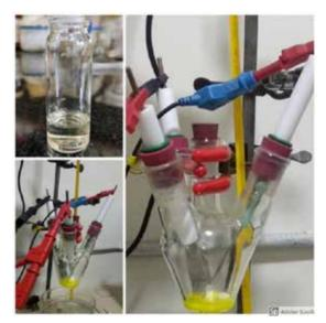
*Figure.* 1: Electrochemical gas tight cell developed in order to maintain inert atmosphere for the electrochemical study of aluminium
