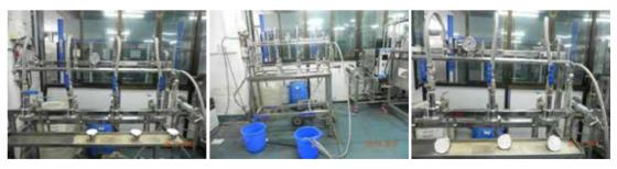
Nanofiltration test skid at Desalination Division, BARC
